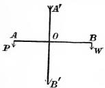
Suppose the lever to be a straight lever AB, having its arms AO = a, and BO = b, and to be acted on by forces P and W perpendicular to the arms.
